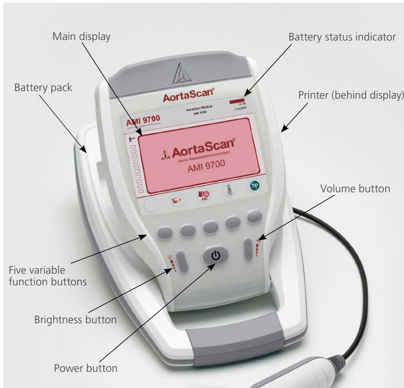
Figure 3. Console Components
